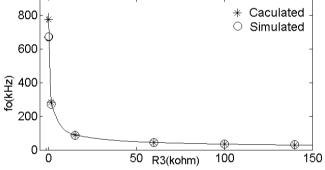
Fig 4: Single Resistor Frequency Control of Proposed Circuit 1
