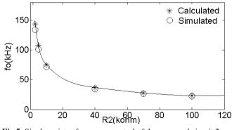
Fig.5: Single resistor frequency control of the proposed circuit 2
