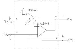
**Fig.2**. Implementation of CDBA using commercially available AD-844 type CFOAs [8]
